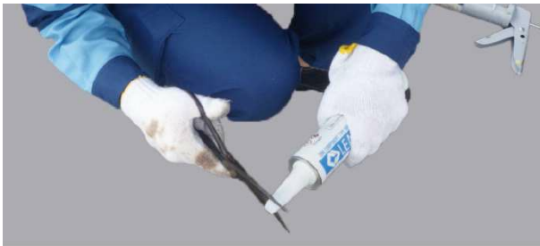
2) Cut the nozzle at the appropriate position
