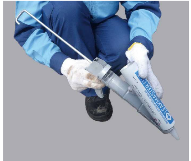
4) Set the cartridge to a caulking gun
