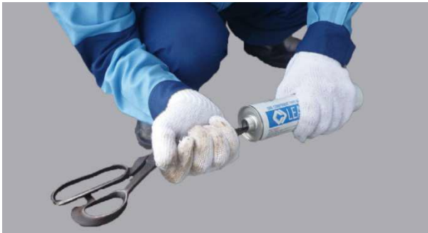
1) Break the moisture-proofing aluminum foil on the top of the cartridge
